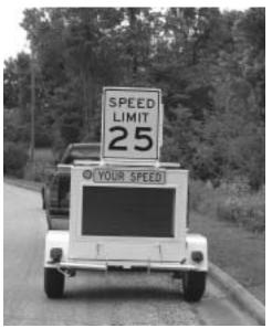
The new radar display uses solar power and the latest in light emitting diode (LED) technology to display messages to drivers. The radar will detect a vehicle's speed, record the speed, and display the speed, along with a message reading "Too Fast" or "Slow Down" depending on the vehicle's speed.
